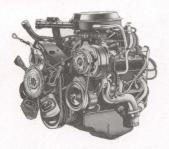
**NEW VORTEC GAS ENGINE** Full-size gasolineengine GMC models have a new standard V6 engine that provides more horsepower and torque than the 4.1 liter engine it replaces. The 4.3 liter V6 Vortec gas engine has a high 9.3 to 1 compression ratio. Swirl inlet ports provide good fuel/air mix, and Electronic Spark Control helps control spark knock.
